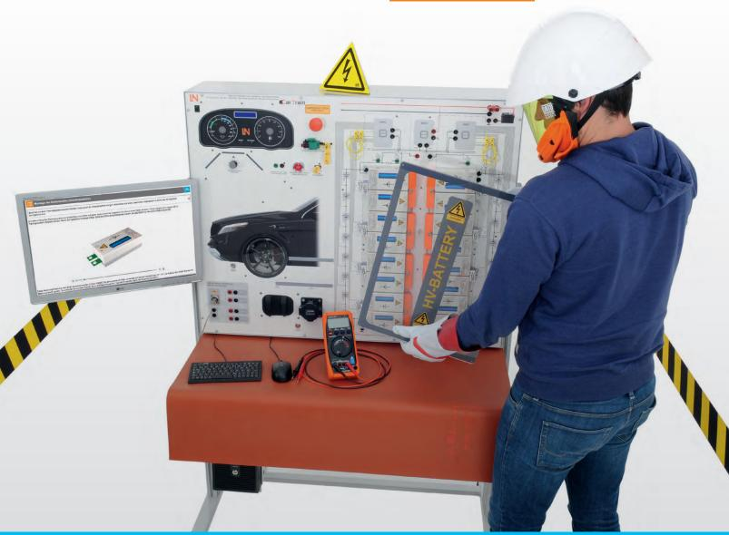
In combination with the personal protective equipment and the integrated high-voltage diagnostic unit, this very practically oriented training system supports in-depth diagnostics unlike any other. with safety clothing and equipment, plus the high-voltage diagnostic tester, the training system provides unique diagnostic range closely aligned to authentic practice.
