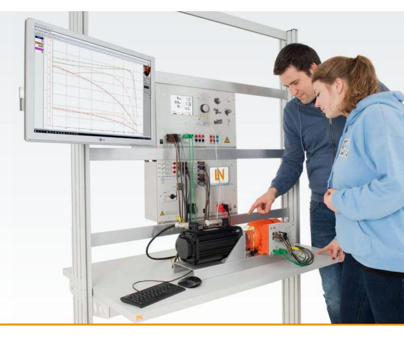
The servo machine testing system permits hands-on investigations of standard industrial drives. In addition to pure drives and brakes, you can also use this system to realistically emulate working machine models. Thus, you can investigate in the lab how machines, generators and drives operate under realistic conditions. In the process, the system records all the important measurement data and displays it in a clear and precise way.
