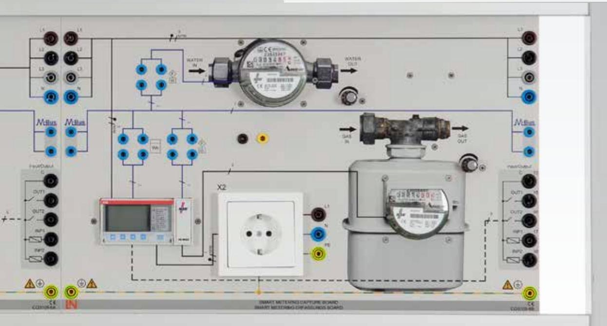
This board can be used as a supplementary addition to a smart metering system. It includes a single-phase, programmable electricity meter, a pulse converter for conventional meters with a pulse input, as well as water and gas meters. All consumption data can be communicated via a bus system. Data from conventional meters with a pulse output can be converted into bus signals.
