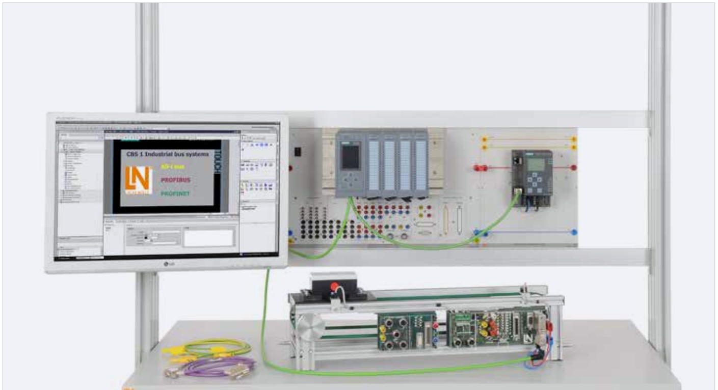
Sample experiment "Industrial bus systems CBS 1"
