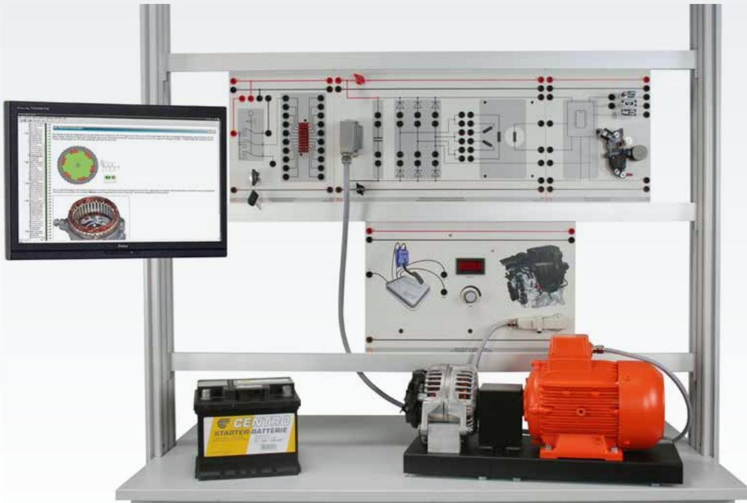
Today's compact generators make use of a monolithic controller. This kind of multifunction controller (MFC) has now largely replaced hybrid controllers. The training system shows how electrical energy is generated in modern vehicles with the help of experiments which build on one another.
