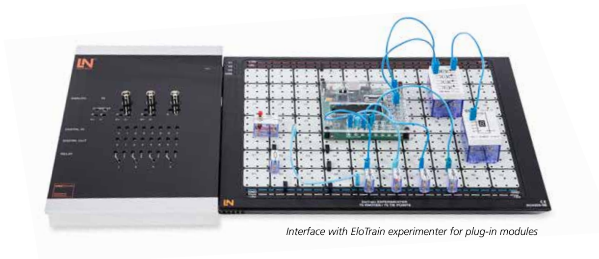
Interface with experimenters hosting experiment cards
